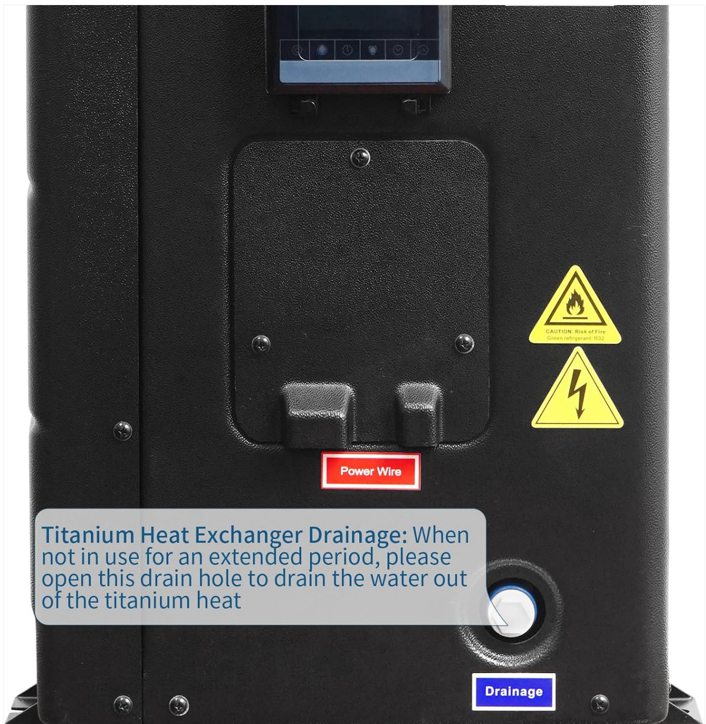
Image: Close-up view of the drainage port on the DOEL Pool Heat Pump, labeled "Drainage". This port is used to drain water from the titanium heat exchanger for maintenance or winterization.
