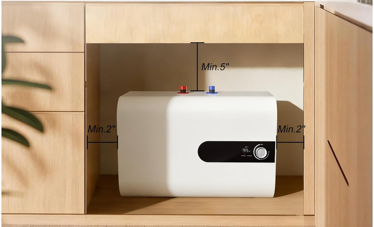
Image 4: Recommended minimum reserved space for under-sink installation, showing clearances of 2 inches on sides/back and 5 inches on top.
