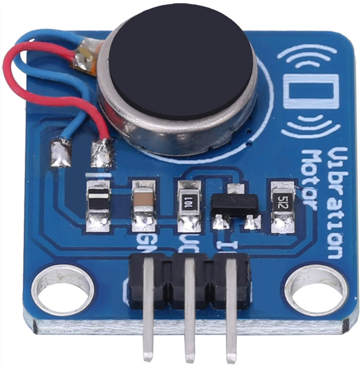
Image description: A top-down view of the Dioche DC5V Vibration Motor Module. The blue circuit board features a circular black vibration motor, resistors, and three connection pins labeled VCC, GND, and IN.
