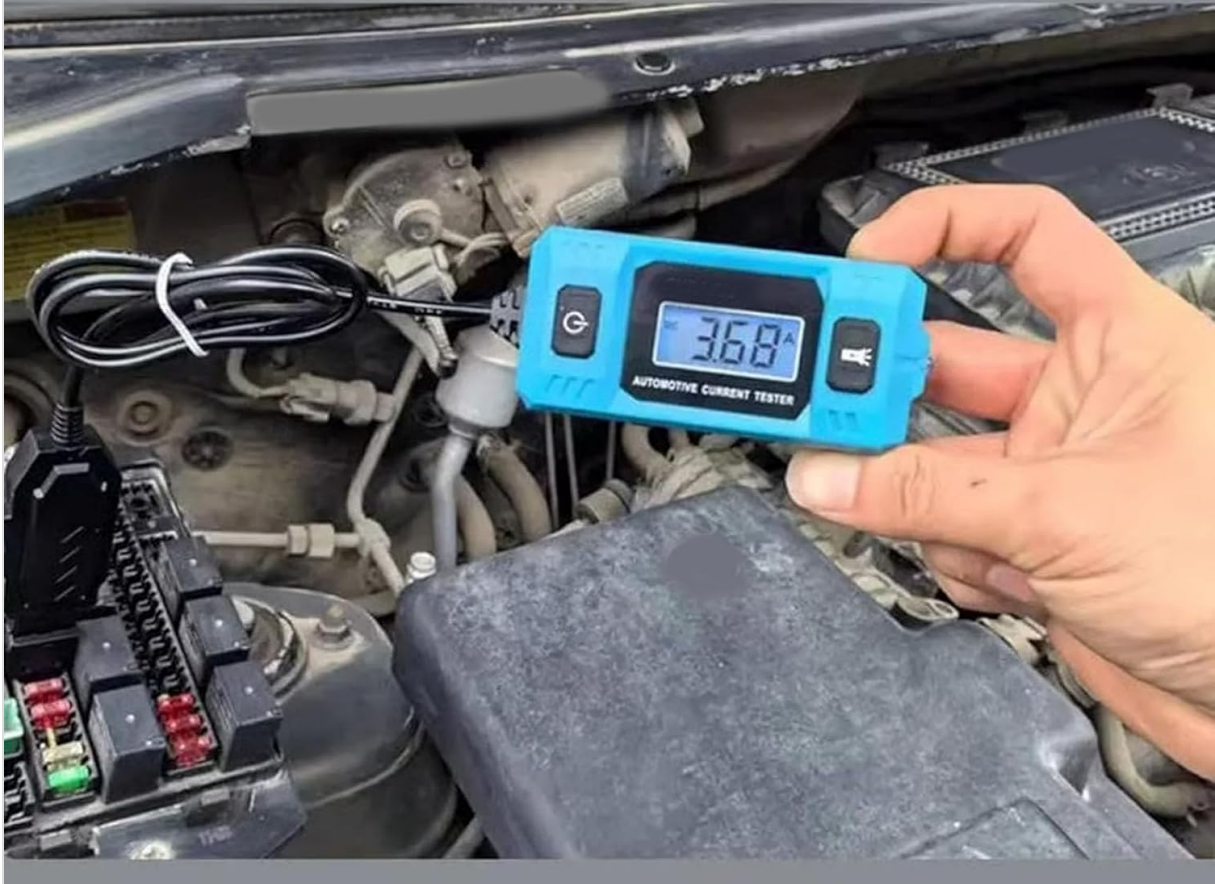
Figure 4: Tester in Operation. This image shows the Cnbj-611 Automotive Current Tester connected to a vehicle's fuse box, actively displaying a current measurement. This demonstrates its use for fault finding in automotive electrical circuits.
