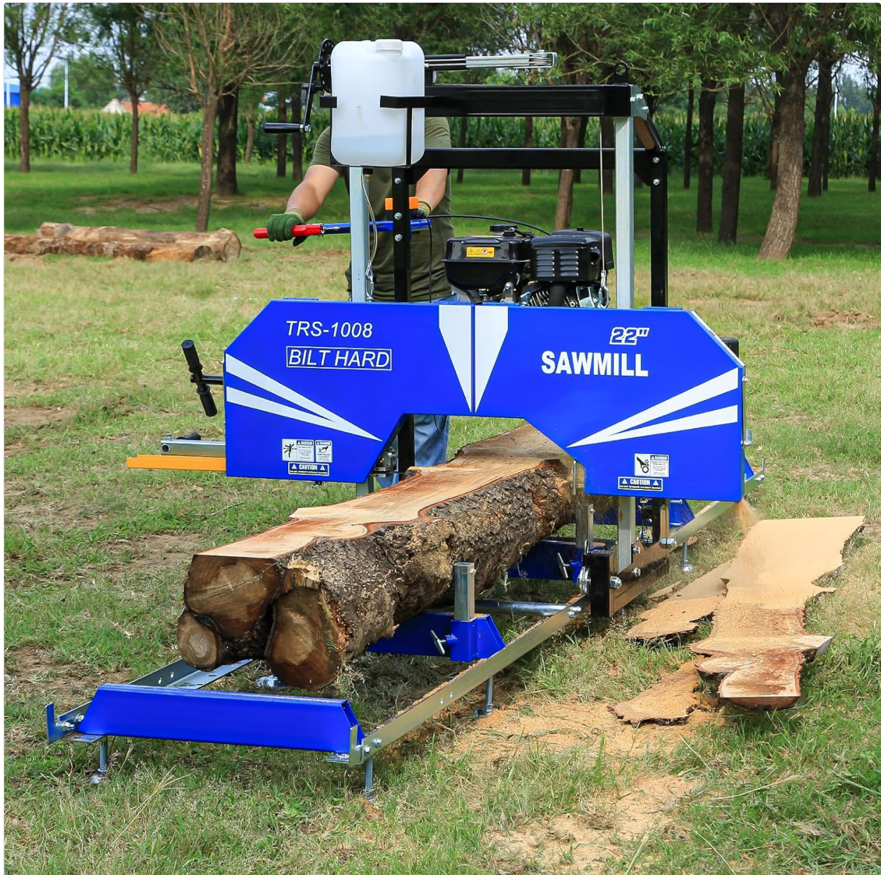
Figure 3: Sawmill fully assembled and ready for operation.
