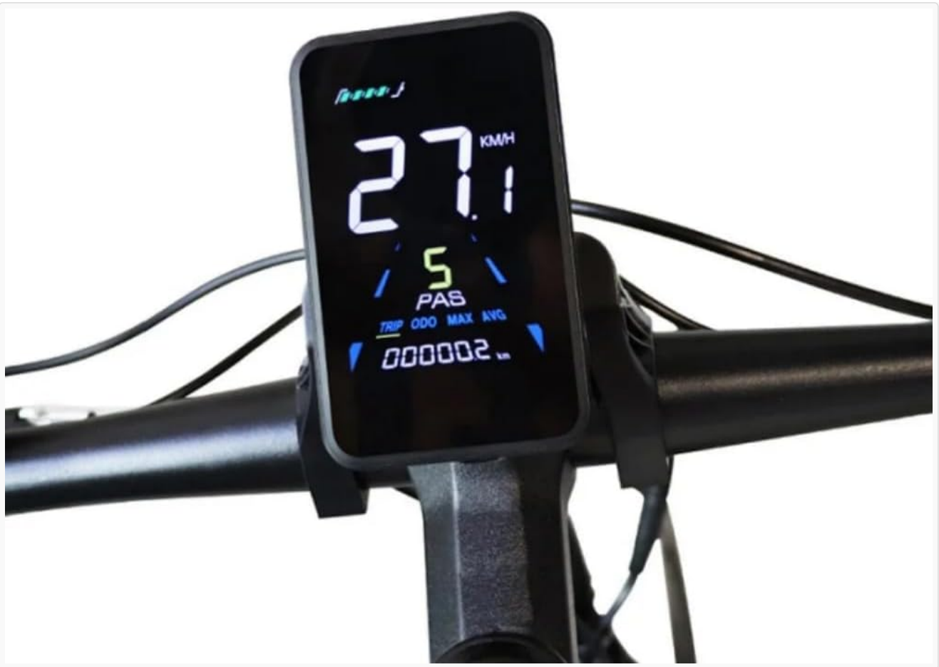
Figure 5.3: The YL81F display correctly mounted on an ebike handlebar.
