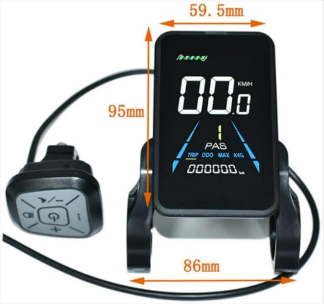
Figure 4.2: Front view of the YL81F display unit with approximate dimensions (59.5mm width, 95mm height, 86mm mount width).
