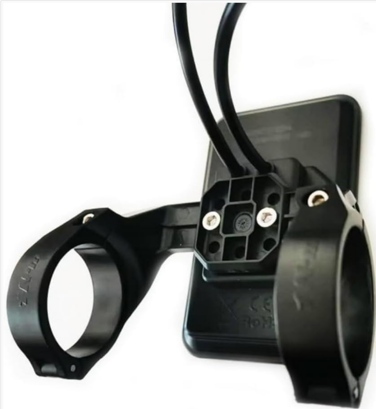
Figure 5.1: Rear view of the display mount, showing attachment points for the handlebar.
