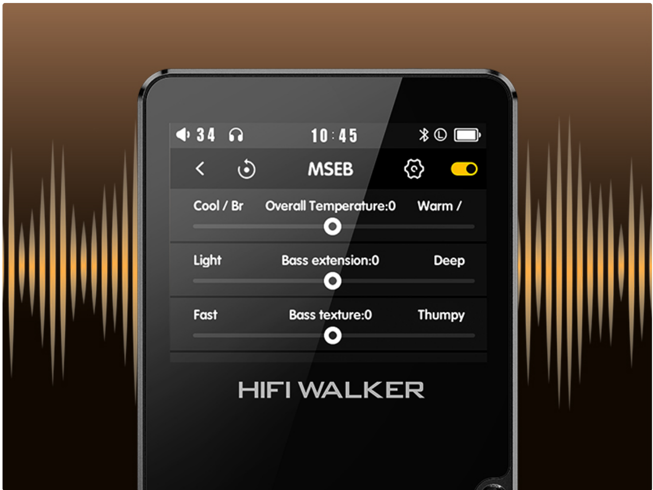
The MSEB equalizer interface on the HIFI WALKER H2 Touch, allowing detailed sound customization.
