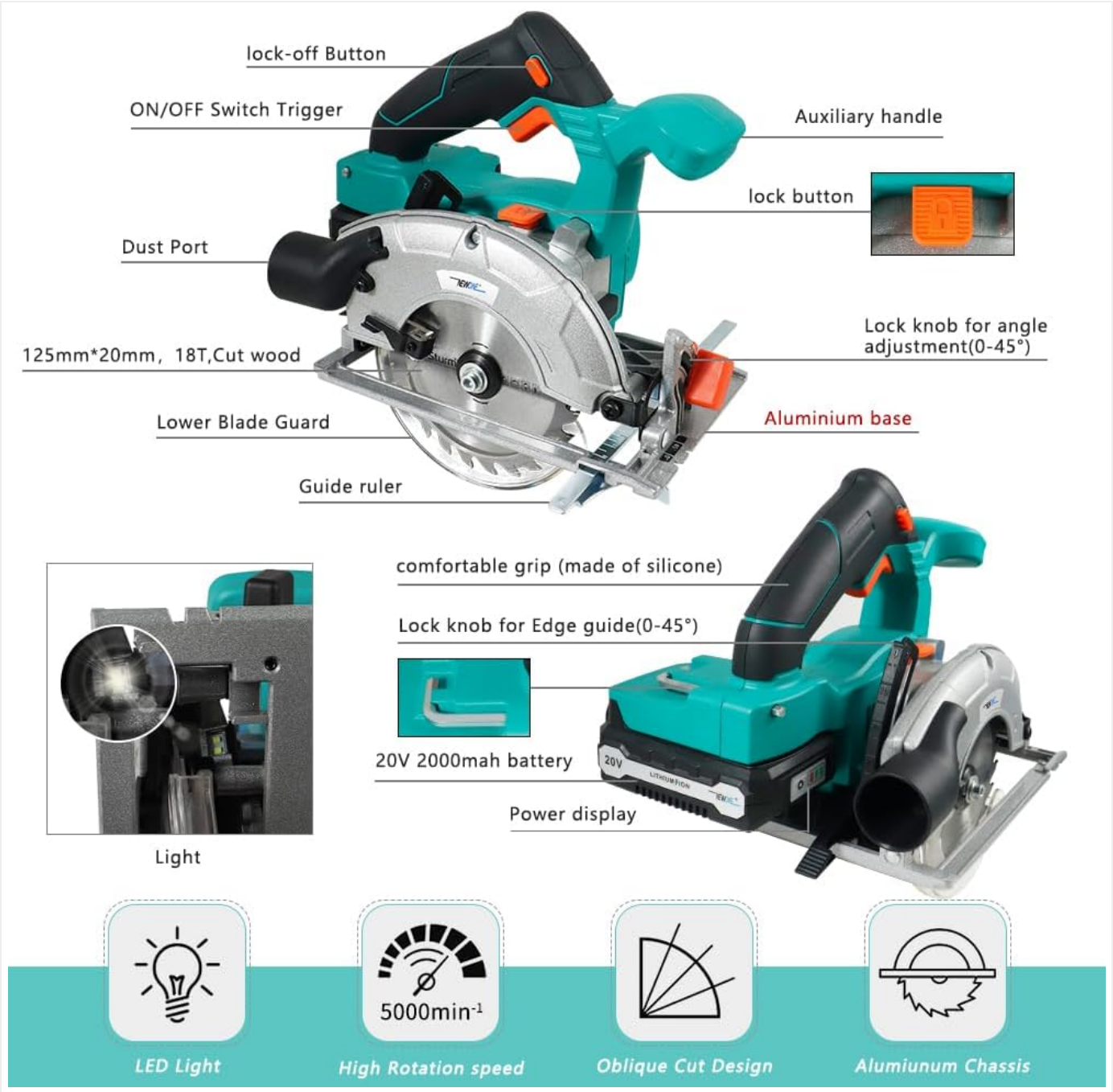
Figure 2.1: Labeled components of the NEWONE 20V Cordless Circular Saw.
