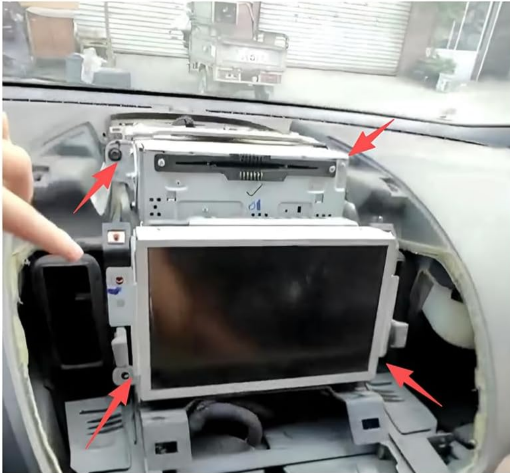
Image: Steps for removing the original CD unit in high-trim models.
