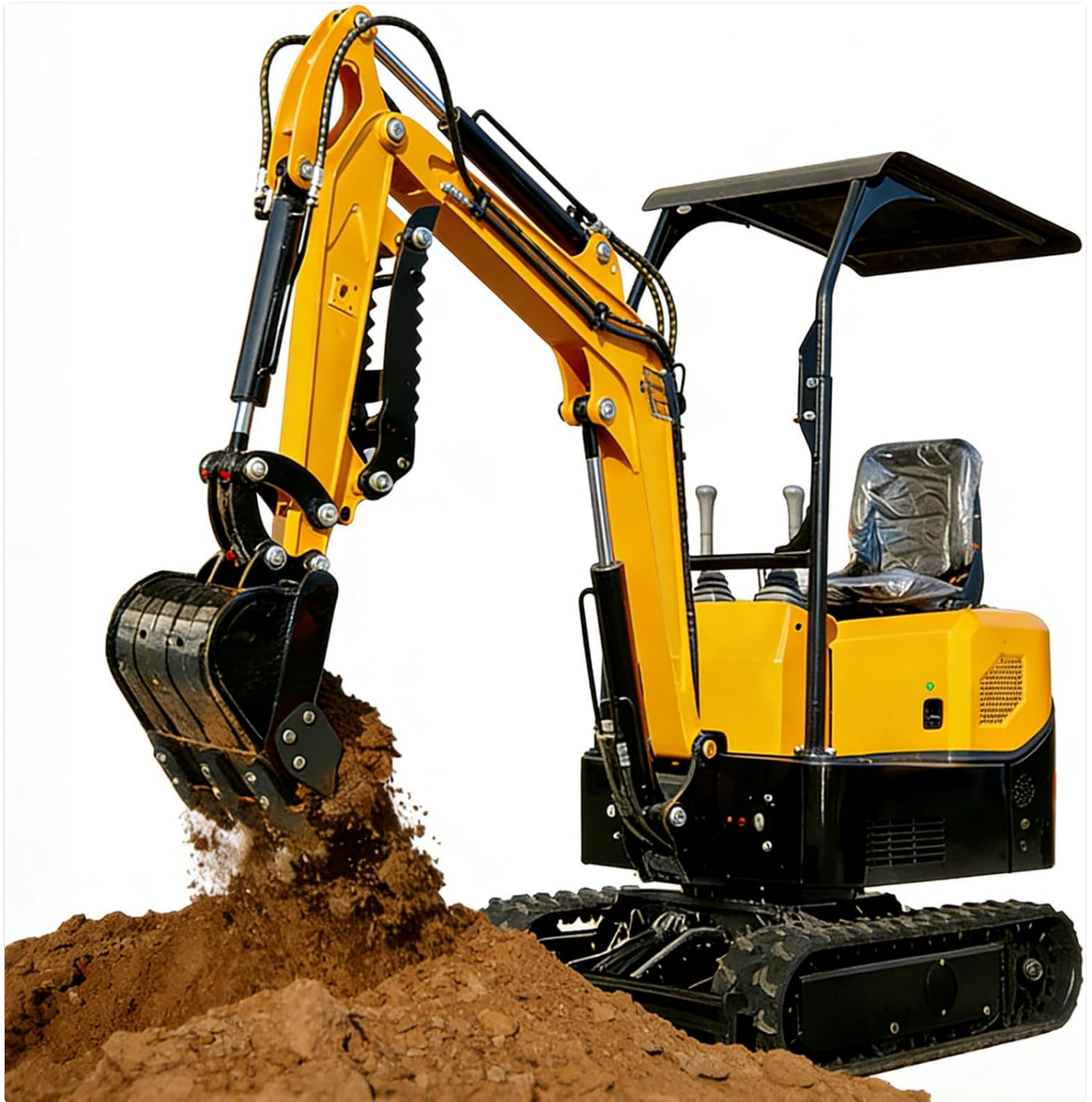
Figure 3.1: Front-side view of the MMS 1 Ton Mini Excavator MS10C, showcasing its compact design and 13.5 HP Briggs & Stratton gasoline engine.
