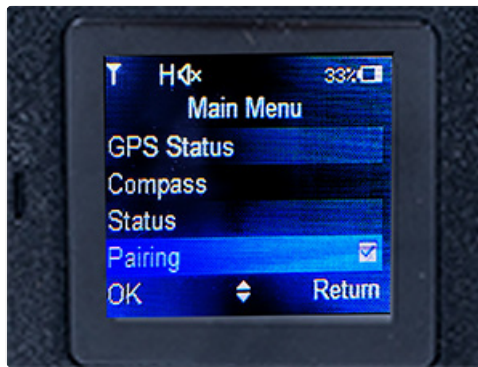
Image: The BS-50 display showing the main menu with 'GPS Status' and 'Pairing' options highlighted.
