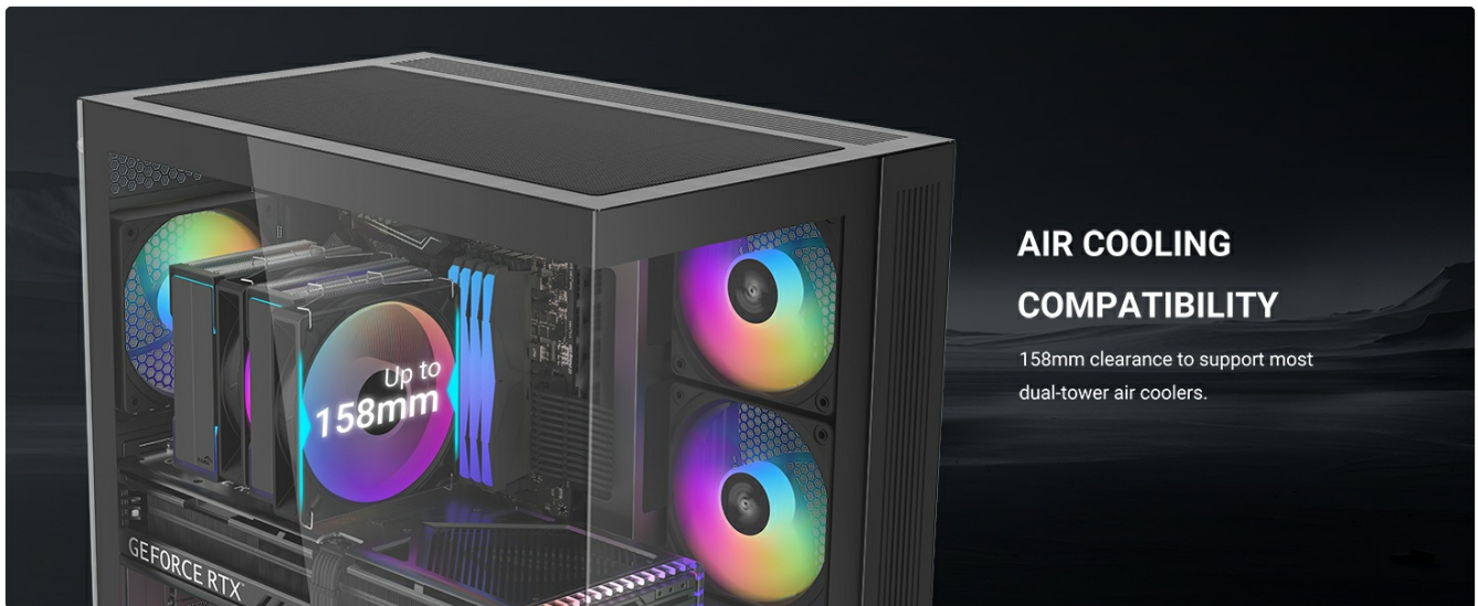
Image 5.7.1: Illustration of the 158mm clearance for CPU air coolers, accommodating most dual-tower air coolers.
