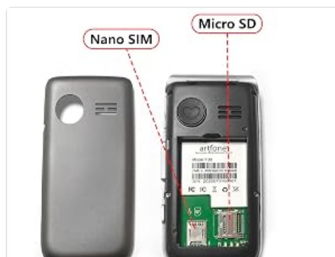
Image: An internal view of the artfone F30 with the back cover removed, clearly showing the slots for Nano SIM and Micro SD cards for installation.
