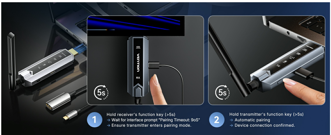
Image 4.2: Instructions for re-pairing the transmitter and receiver units.
