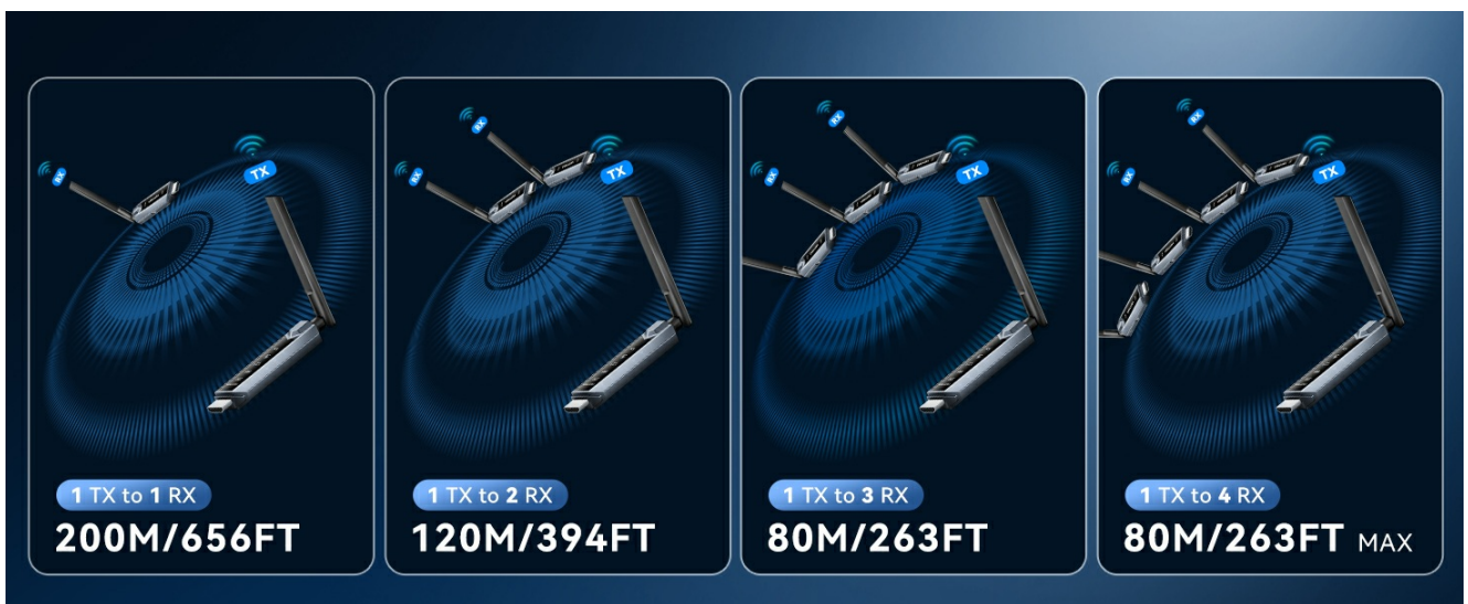
Image 3.3: Diagram showing transmission distances with multiple receivers (1TX to 1RX, 2RX, 3RX, 4RX).
