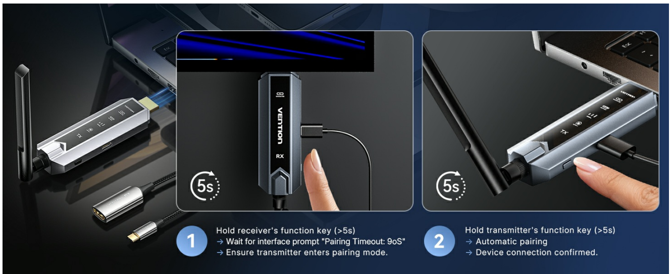
Image 4.1: Visual guide for connecting the transmitter and receiver units.
