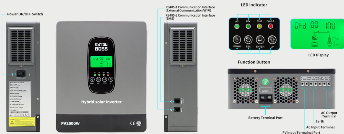
Figure 3.2: Detailed view of the inverter's front panel, side ports, and rear connections. This image highlights the Power ON/OFF Switch, RS485-1 and RS485-2 communication interfaces, LED indicators (AC, INV, CHG, FAULT), LCD Display, Function Buttons (DOWN, ESC, ENTER, UP), Battery Terminal Port, AC Output Terminal, Earth Terminal, and PV Input Terminal Port.
