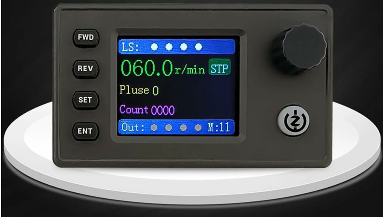
Figure 3.2: The ZK-SMC05 controller's display, emphasizing support for 20 motion modes, expansion buttons, limit switches, output control, and display in both Chinese and English.
