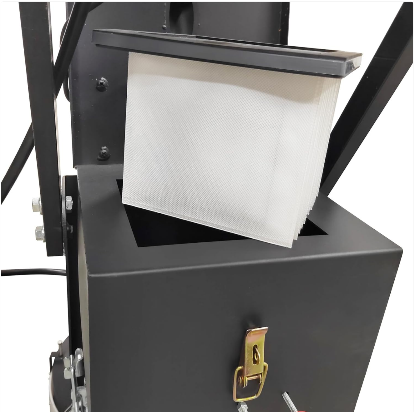
Figure 6: Detail of the filter element within the dust collection system.
