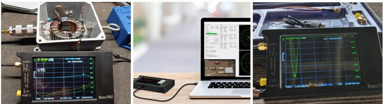
Image: The NanoVNA-H4 connected to a laptop running NanoVNASaver software and an Android phone, demonstrating PC and Android control capabilities.
