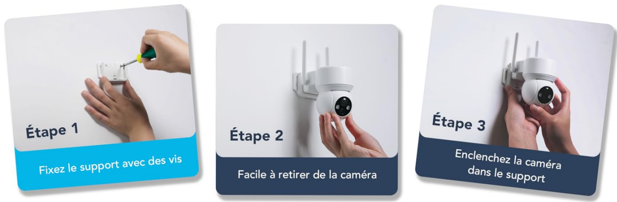
Figure 4.2: Simple three-step installation process for the GNCC W30 camera.
