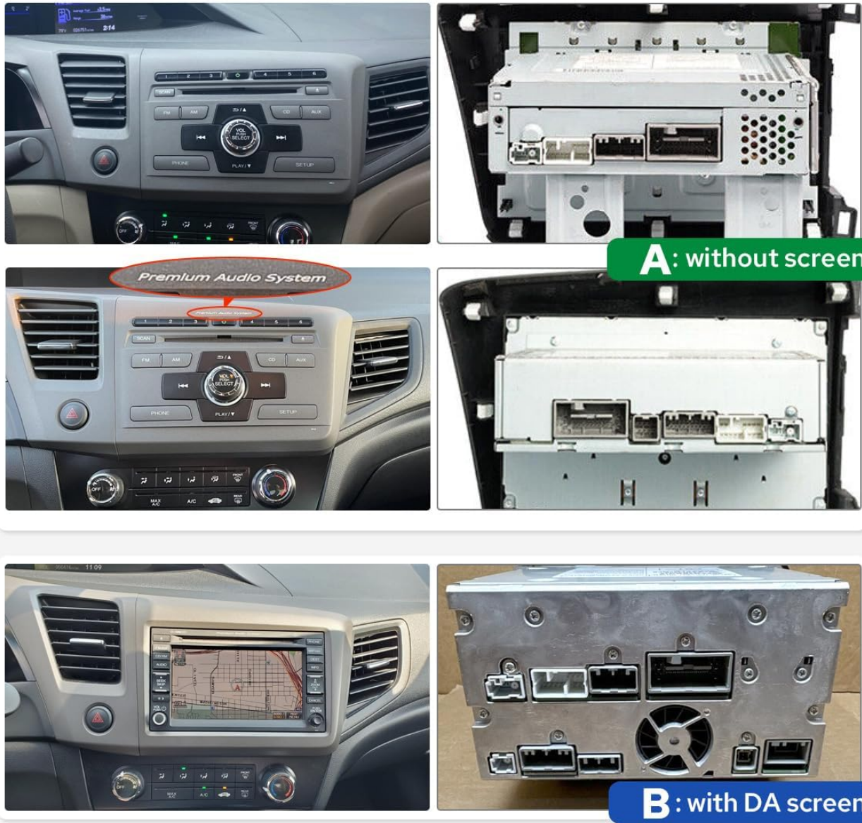
Figure 1: Confirming Car Dashboard Type. This image illustrates two common dashboard configurations for the Honda Civic 2012, labeled 'A: without screen' and 'B: with DA screen', to help identify the correct wiring harness for your vehicle.
