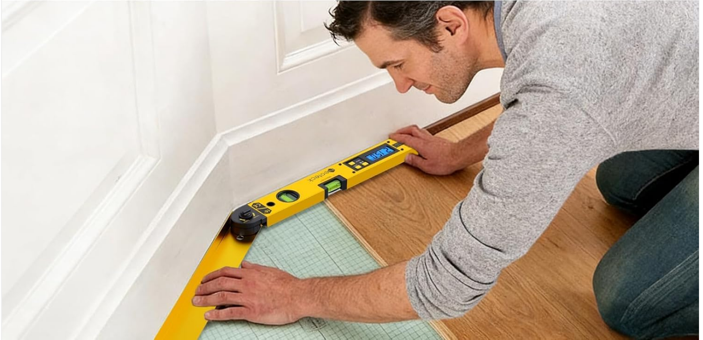
Image: The angle finder displaying a 45° angle, illustrating its 0-225° measuring range.
