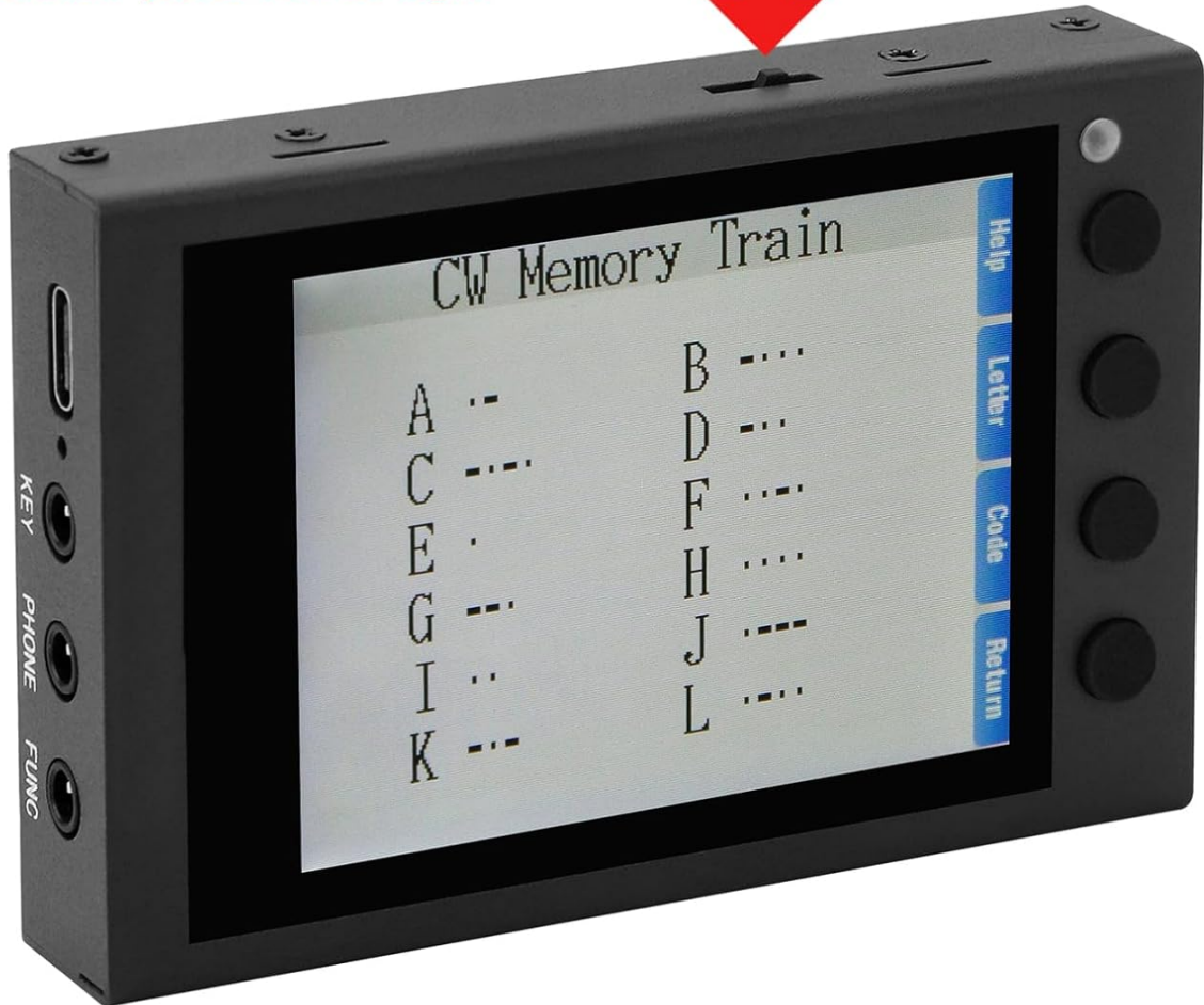
Figure 3: Front view of the HAMCUBE PRO displaying Morse code characters on its screen.
