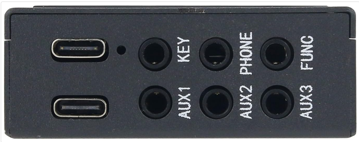
Figure 2: Side view showing the various input/output ports for external connections.
