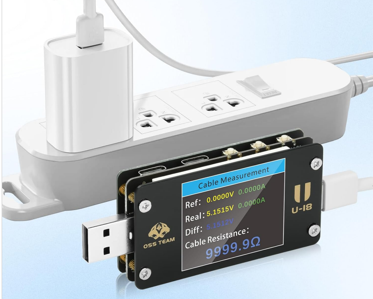
Figure 4: The tester performing a wire internal resistance measurement, displaying reference voltage/current, real voltage/current, difference, and calculated cable resistance.
