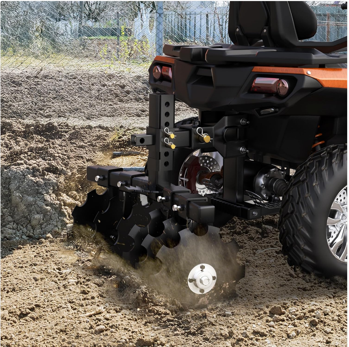
Image: The disc plow harrow connected to a vehicle, illustrating its use for soil preparation.
