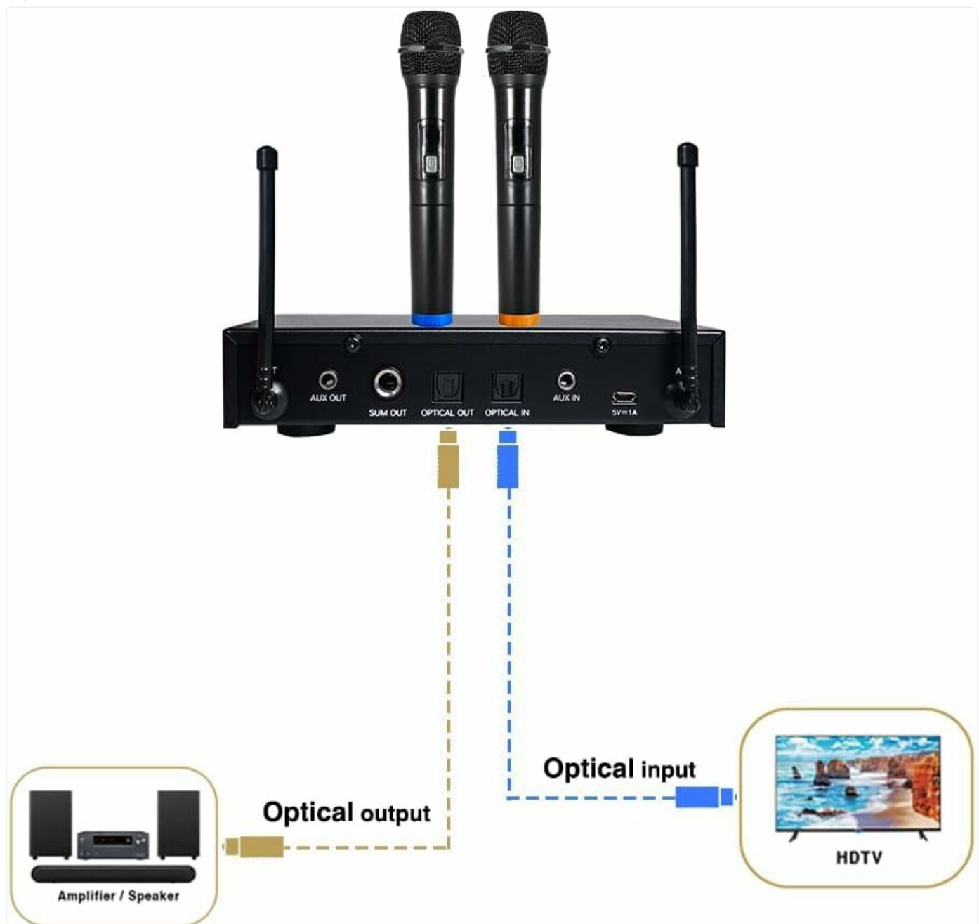
Image: Connection Diagram 1: Optical Connection. Illustrates connecting the TV's optical output to the receiver's optical input, and the
