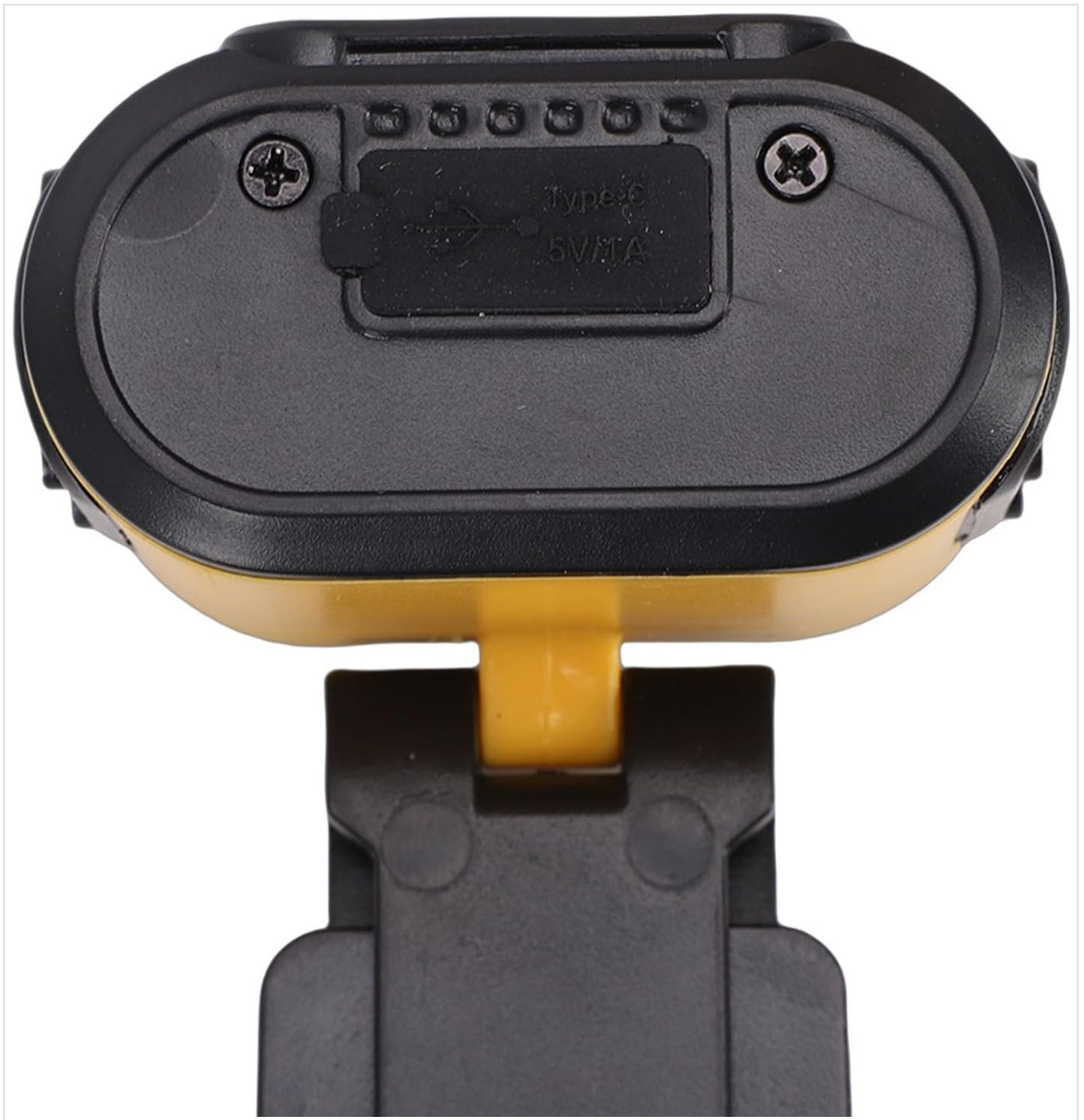
Image: A close-up view of the camera's top, showing the Type-C charging port and indicator lights.
