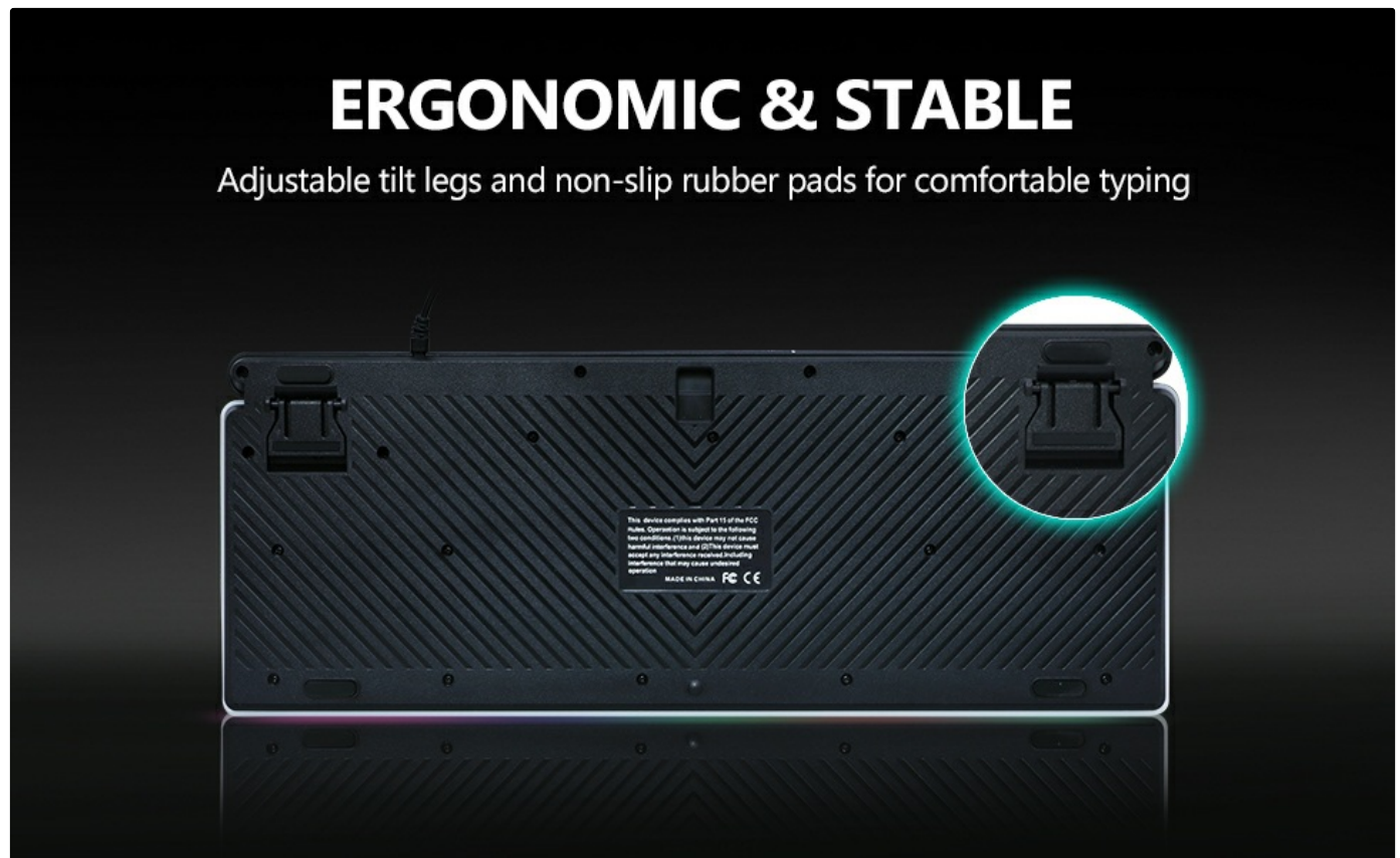
Image 2.1: The underside of the keyboard with a close-up of the adjustable tilt legs, which can be extended for an angled typing position.
