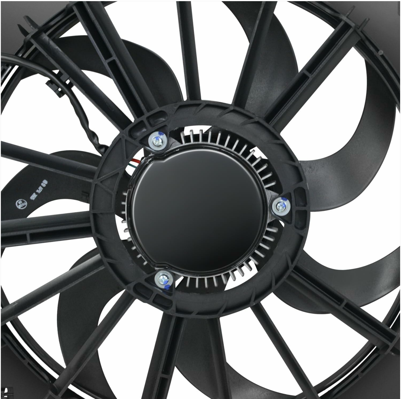
Image 6.1: Close-up of the fan blades, useful for visual inspection of potential damage or debris.
