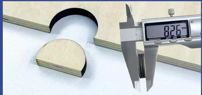
8mm basswood plywood in one pass
