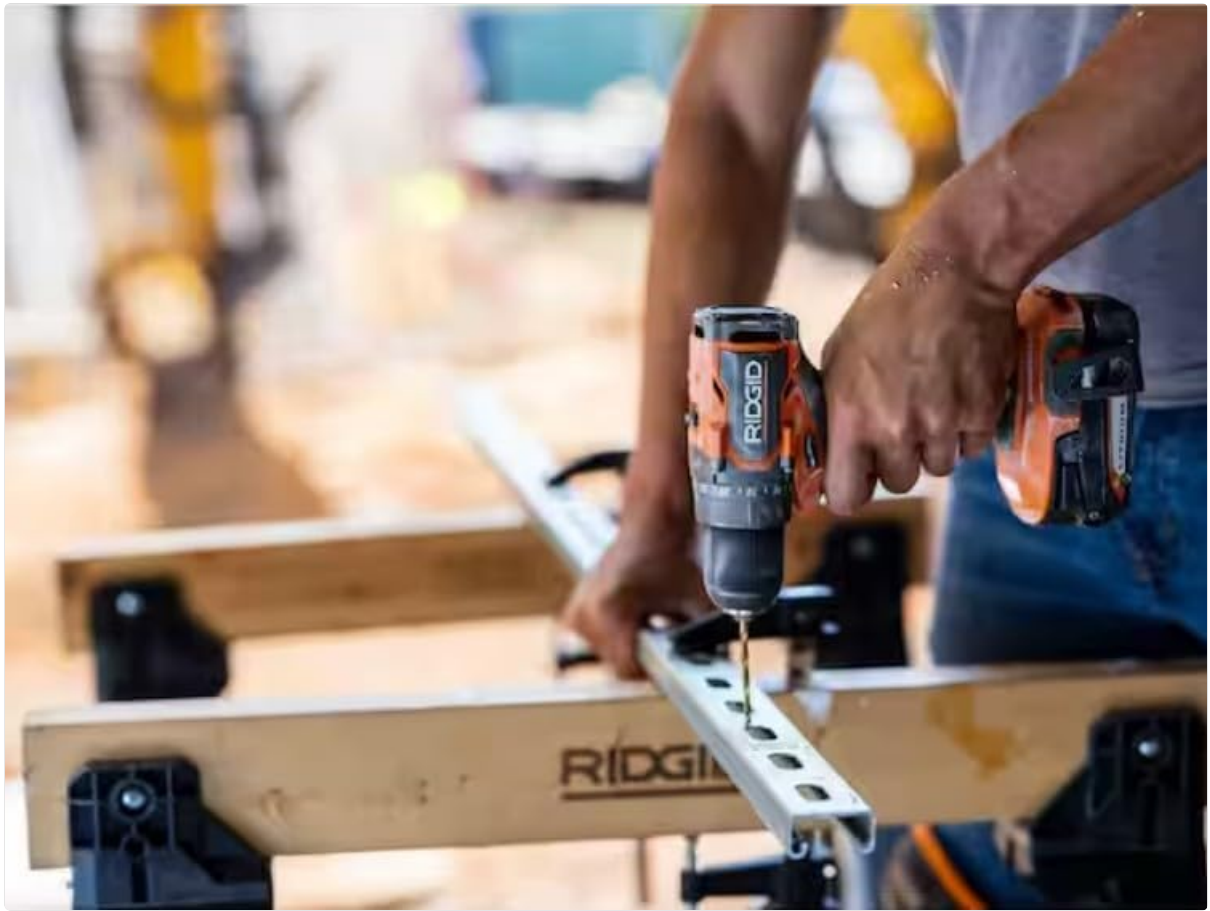
Figure 8: Drilling into a metal channel.
