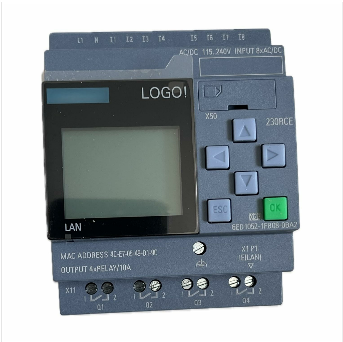
Figure 1: Front view of the Generic LOGO! 230RCE Logic Module, showing the display, control buttons, and connection terminals.
