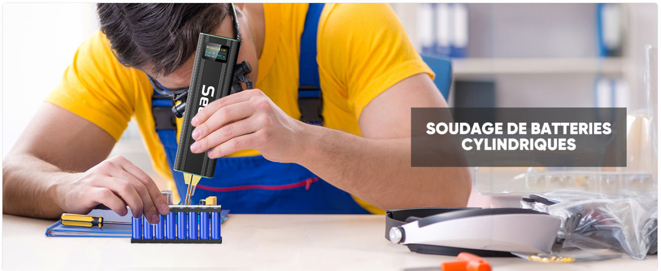
Image 5.3: A technician using the SEESII spot welder to assemble a battery pack.
