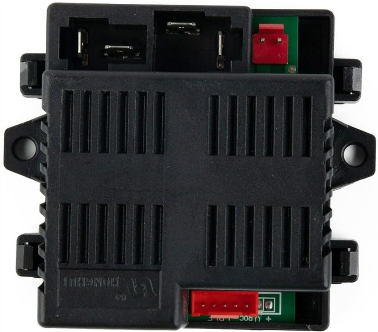
Figure 4.2: Top-down view of the HH-670K-2.4G 12V Receiver. This perspective highlights the ventilation grilles on the top casing and the layout of the connection terminals.
