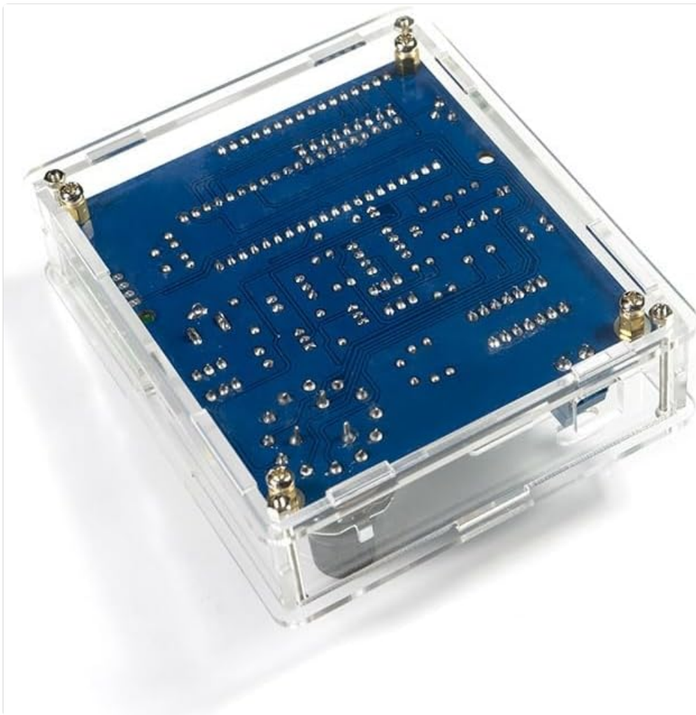
Figure 4: Rear view of the FLC Meter, showing the PCB mounted within the clear acrylic enclosure.
