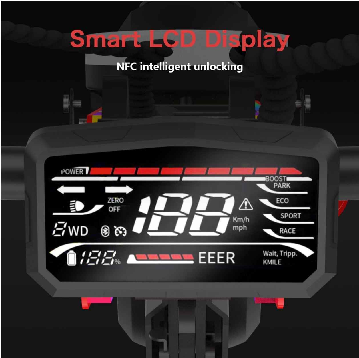
Figure 3: Smart LCD Display with key ride information.
