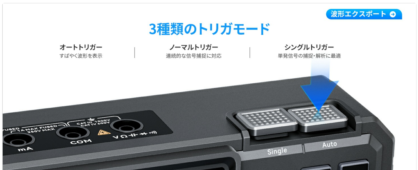
Figure 4.1.2: Trigger mode selection buttons.
