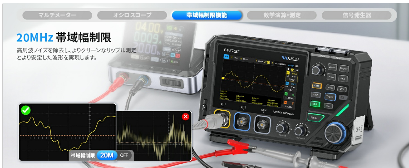
Figure 4.1.3: Effect of 20MHz bandwidth limit on waveform clarity.
