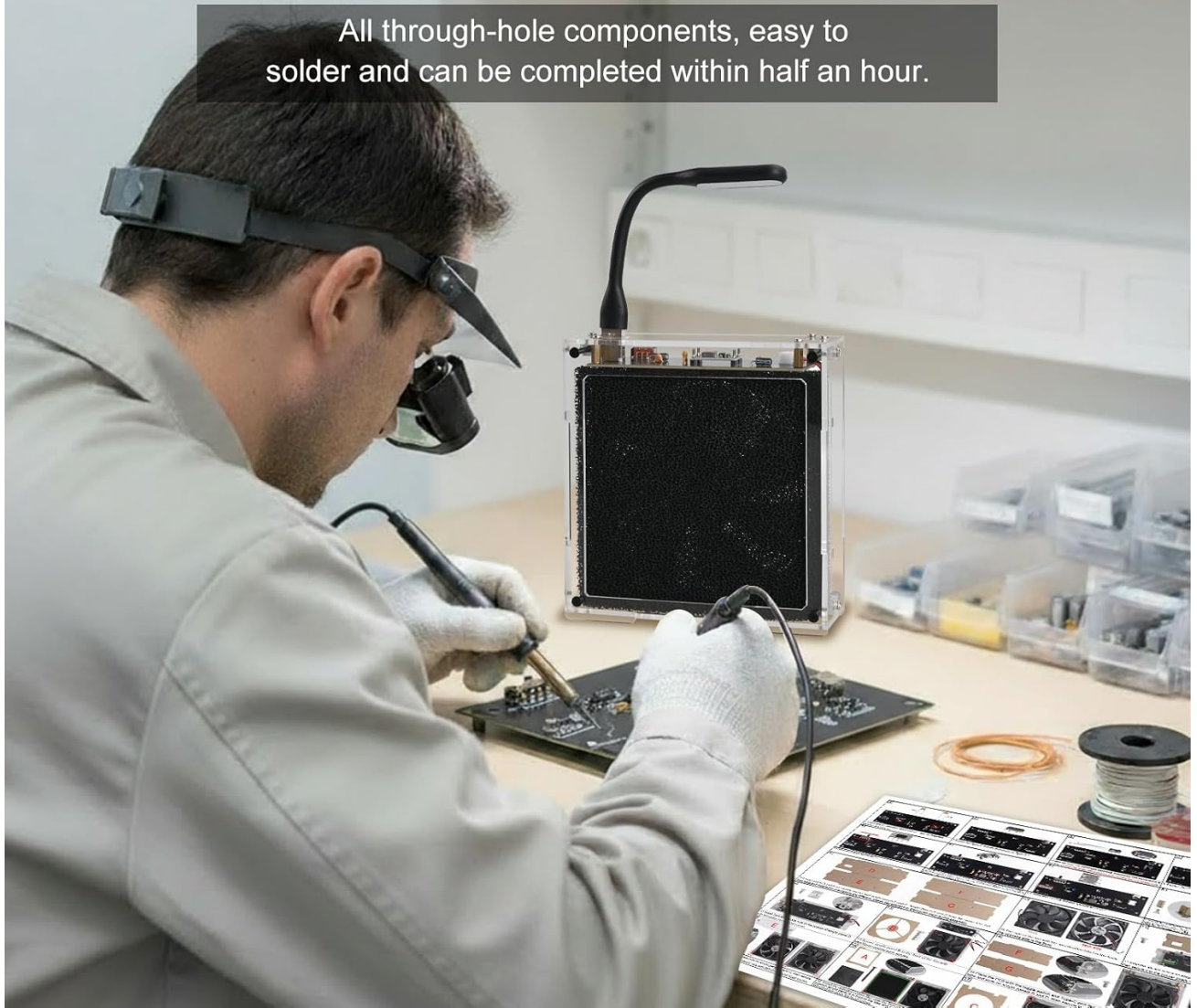
Image 5.2: Solder Fume Extractor Kit Assembly. This image illustrates the assembly of the solder fume extractor kit, emphasizing its through-hole components for easy soldering.
