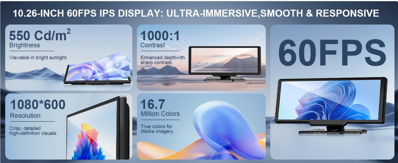
Image: Infographic detailing the 10.26-inch IPS display features: 550 Cd/m 2 brightness, 1000:1 contrast, 1600x600 resolution, 16.7 million colors, and 60FPS refresh rate.
