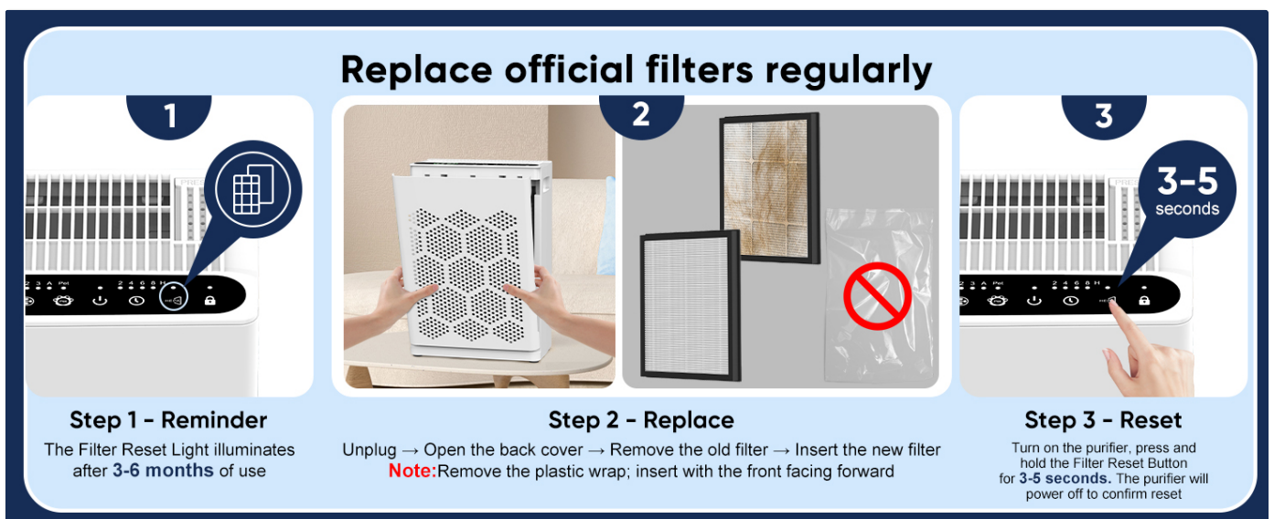
Figure 3.1: Filter removal and installation process.
