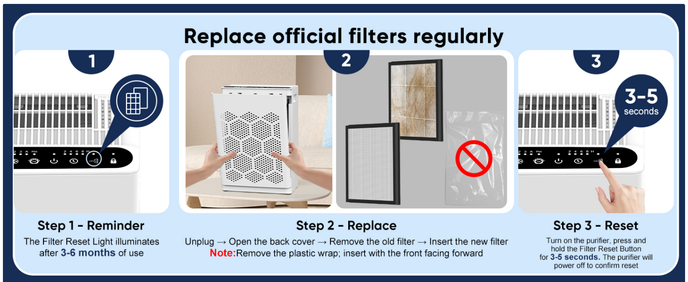
Figure 5.1: Filter replacement steps.
