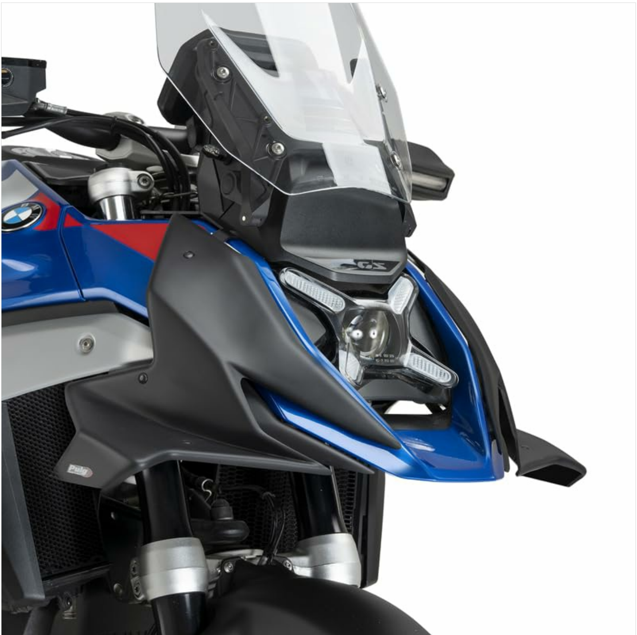
Image 4.3: Front view of the BMW R1300GS showcasing the installed Puig PISTA #5 Front Spoiler.
