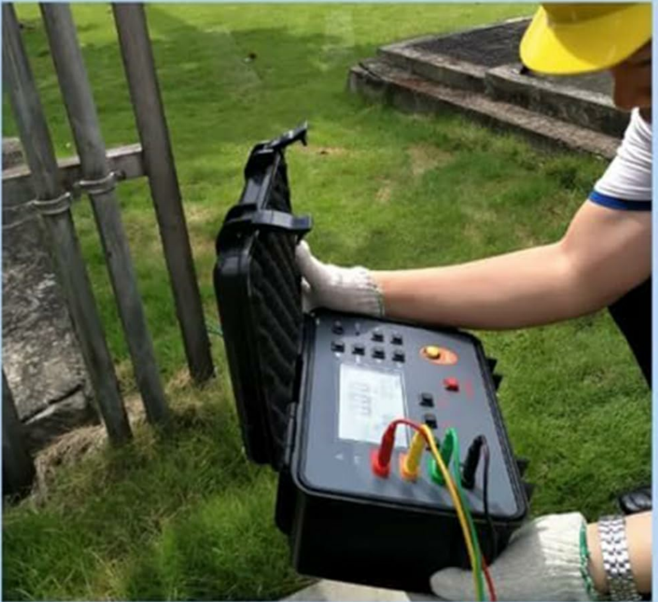
Image 6.2: A user setting up the VTSYIQI Earth Ground Resistance Tester in a field environment, demonstrating the practical application of the device.
