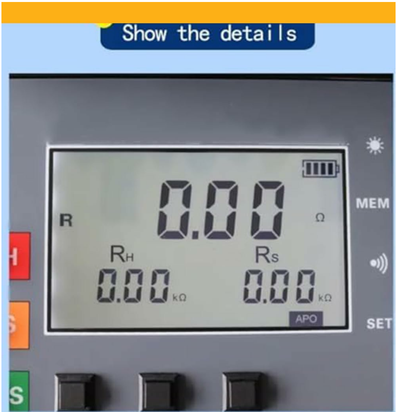
Image 7.2: A close-up view of the tester's LCD display, showing the measured resistance (R) and soil resistivity (R H , R S ) values.
