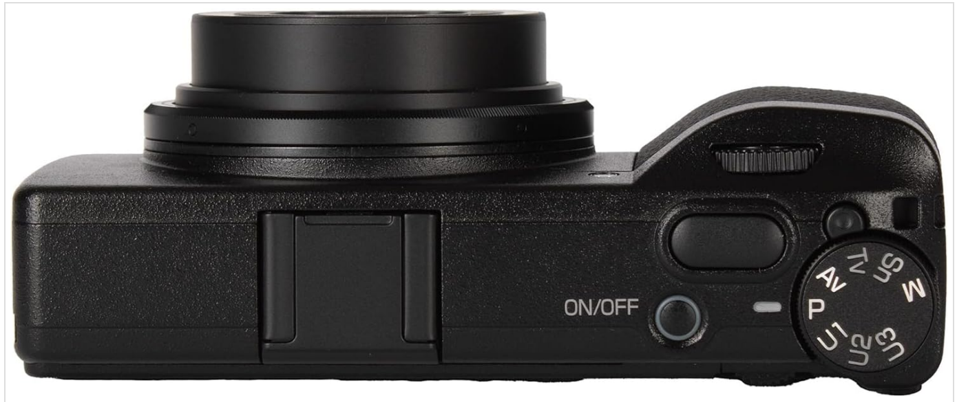
Image: Top view of the Ricoh GR IV camera, highlighting the ON/OFF button and the mode dial for selecting shooting modes.
