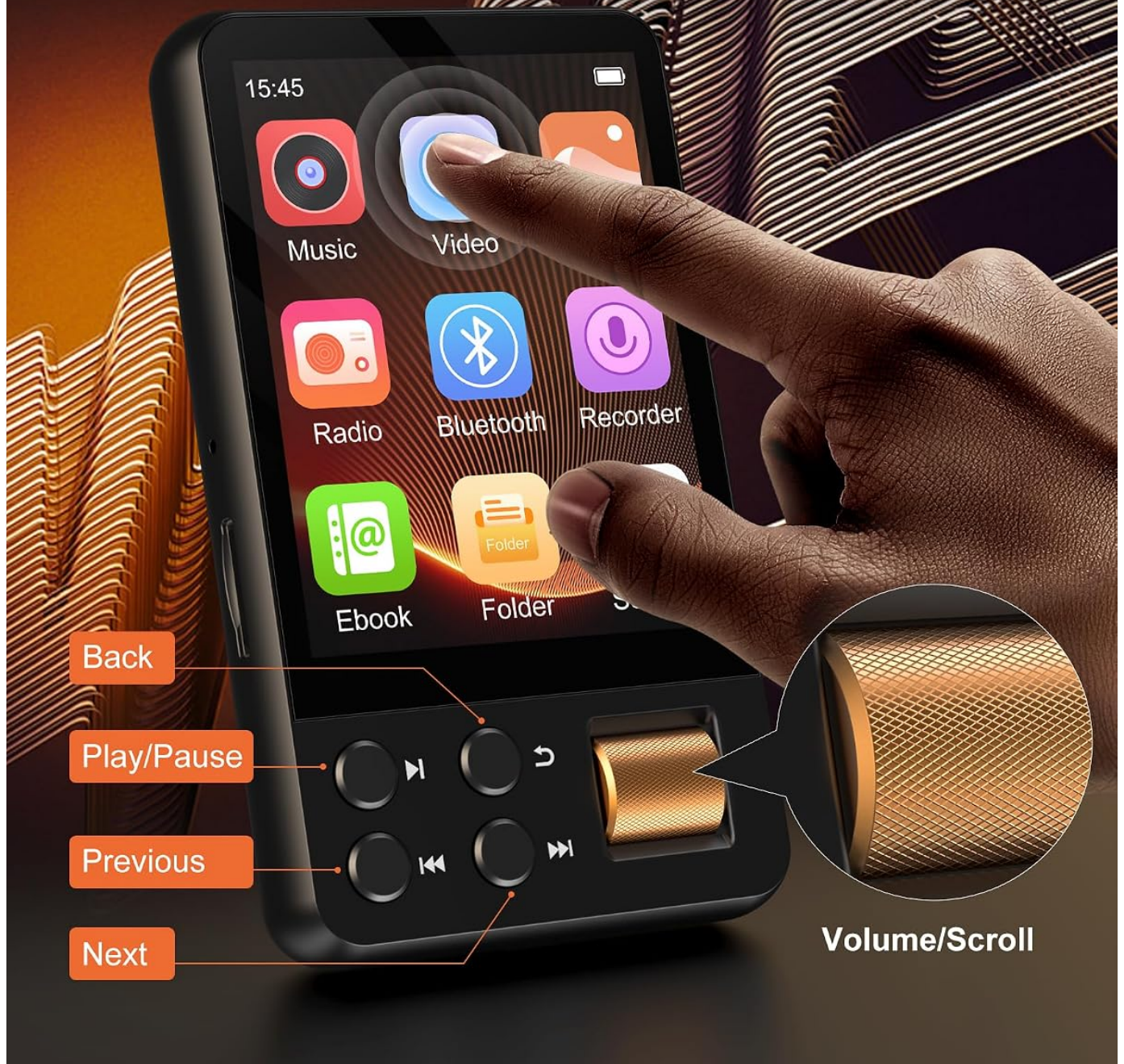
Image: A detailed view of the AGXOV D28 MP3 Player highlighting its touchscreen and physical buttons. Labels indicate functions such as Back, Play/Pause, Previous, Next, and the multi-functional Volume/Scroll knob.
