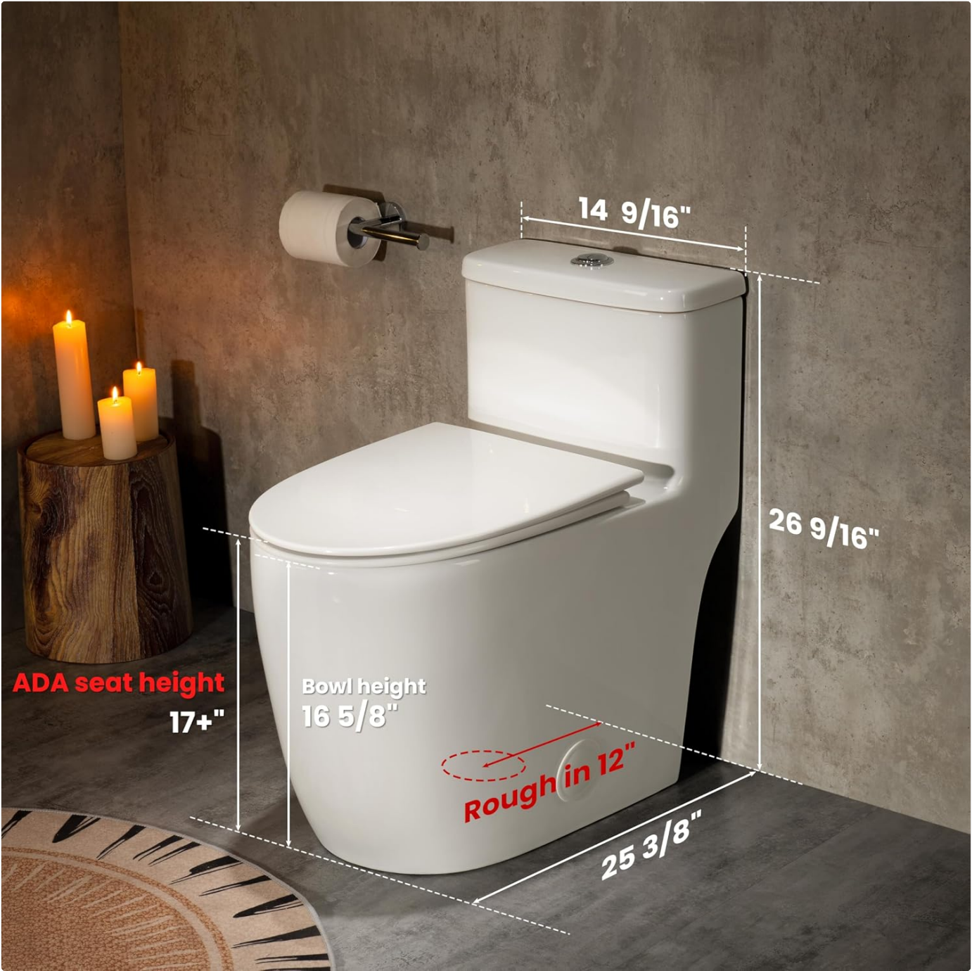
Figure 2: Toilet dimensions and rough-in measurement.
