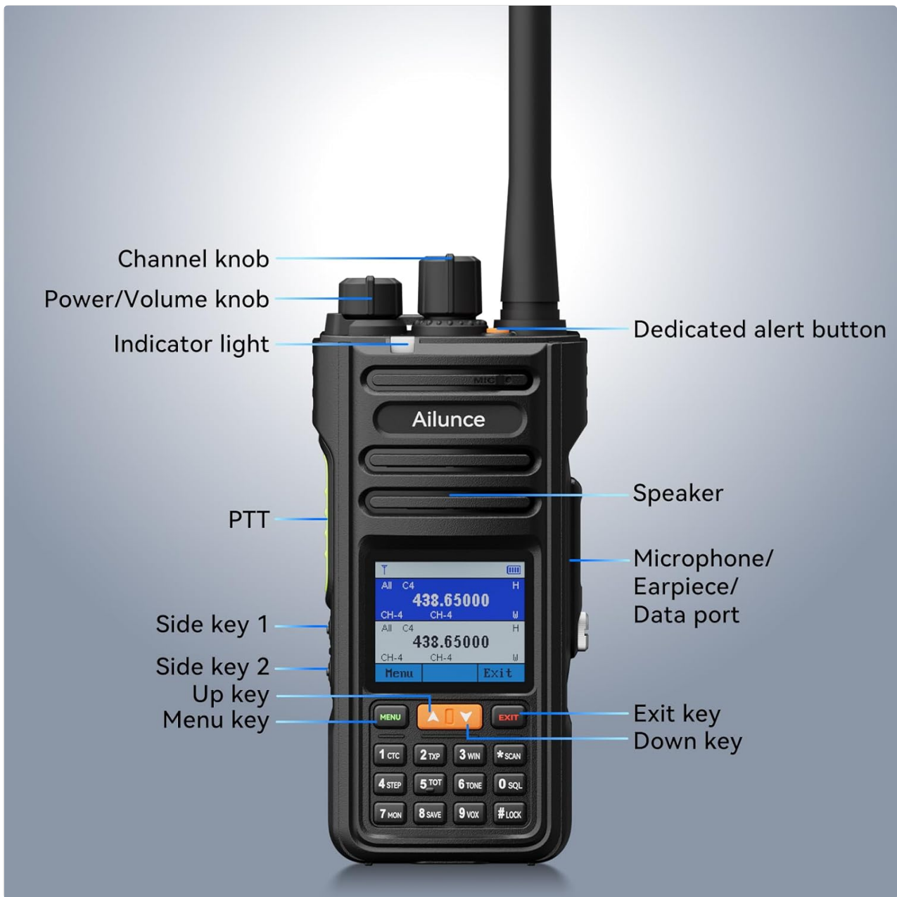
Image: Diagram of the Ailunce HA2 radio with labels pointing to the antenna, indicator light, PTT button, side keys, menu key, exit key, down key, function keys, channel knob, power/volume knob, dedicated alert button, speaker, and microphone/earpiece/data port.
