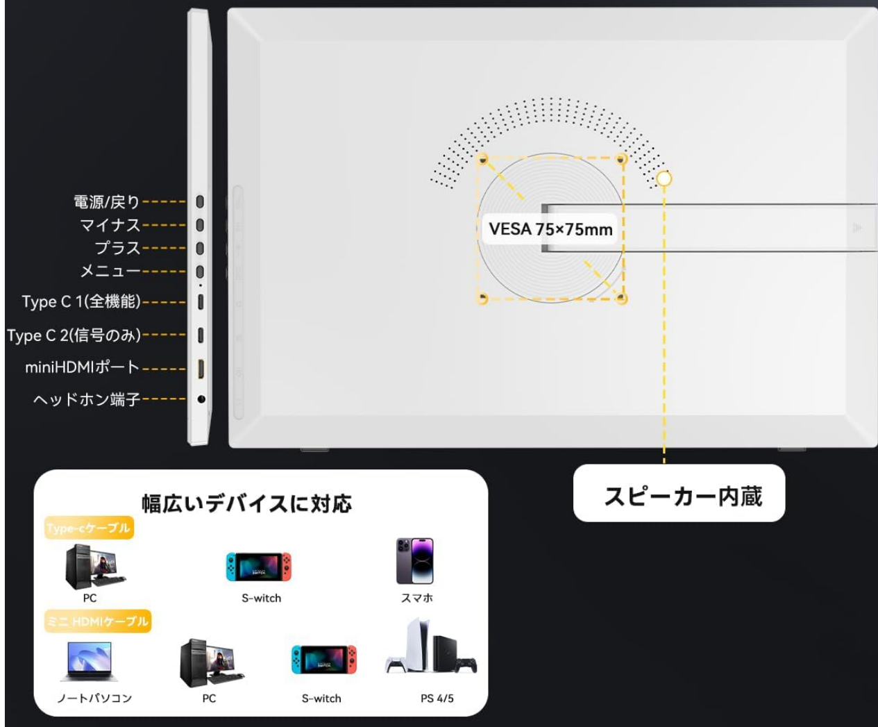
Image 5.2: Overview of monitor ports and various compatible devices.
