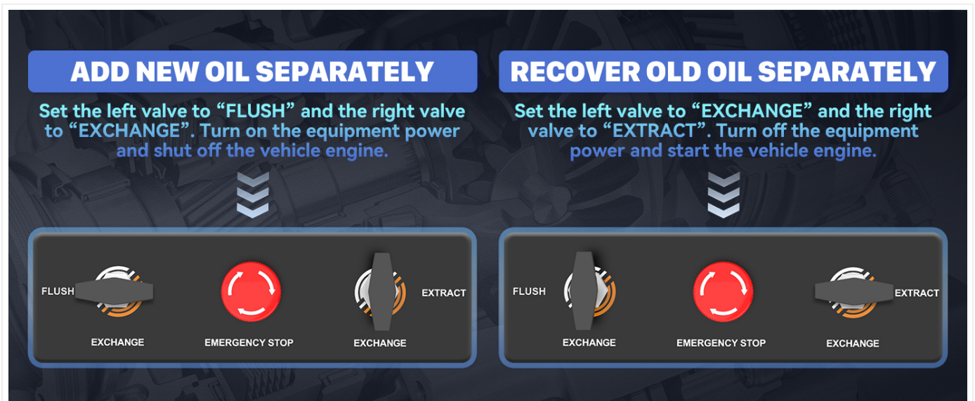
Figure 10: Instructions for draining the new and old oil drums.
