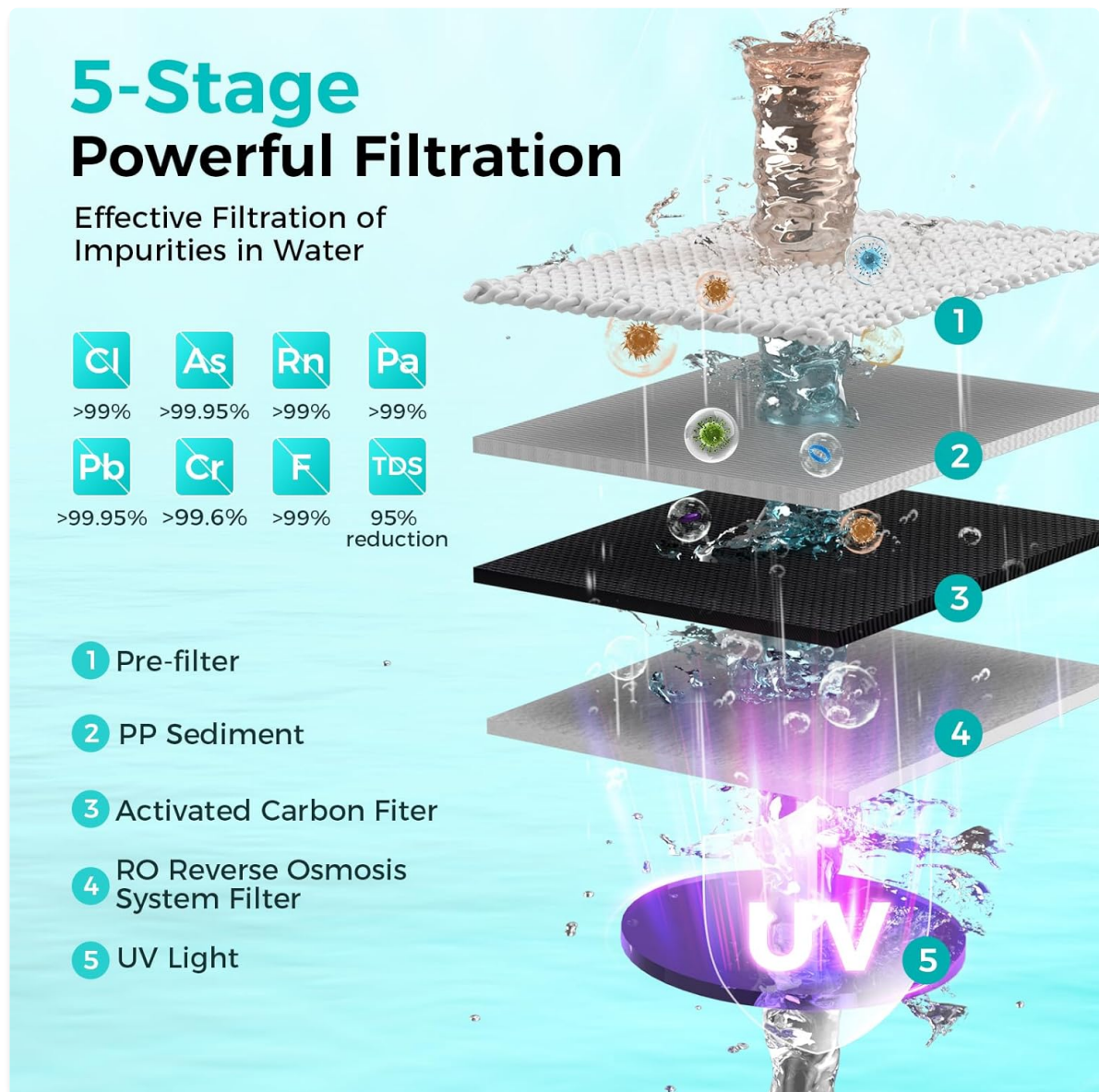
Figure 4: Illustration of the 5-stage filtration process, including Pre-filter, PP Sediment, Activated Carbon Filter, RO Reverse Osmosis System Filter, and UV Light.
