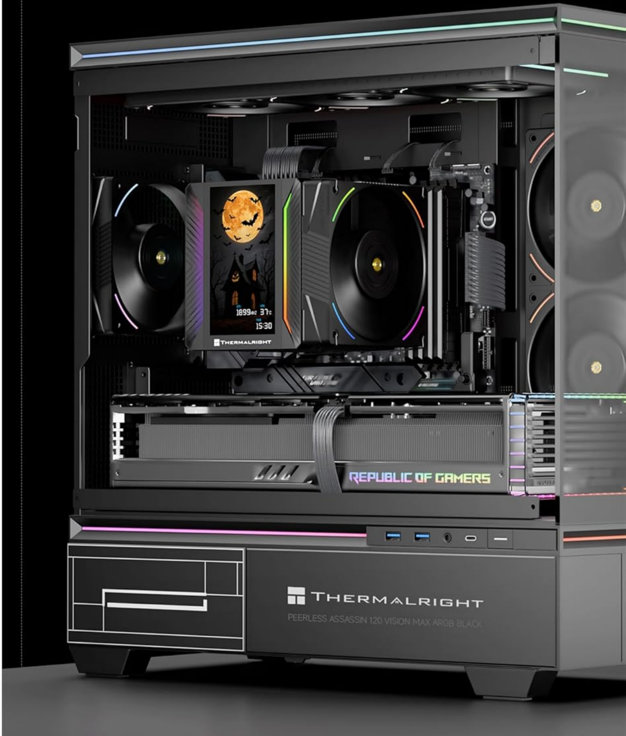
Figure 3: Customizable LCD Display. This image shows the 5-inch IPS LCD screen integrated into the cooler, capable of displaying personalized images, animations, and system data with high quality.
