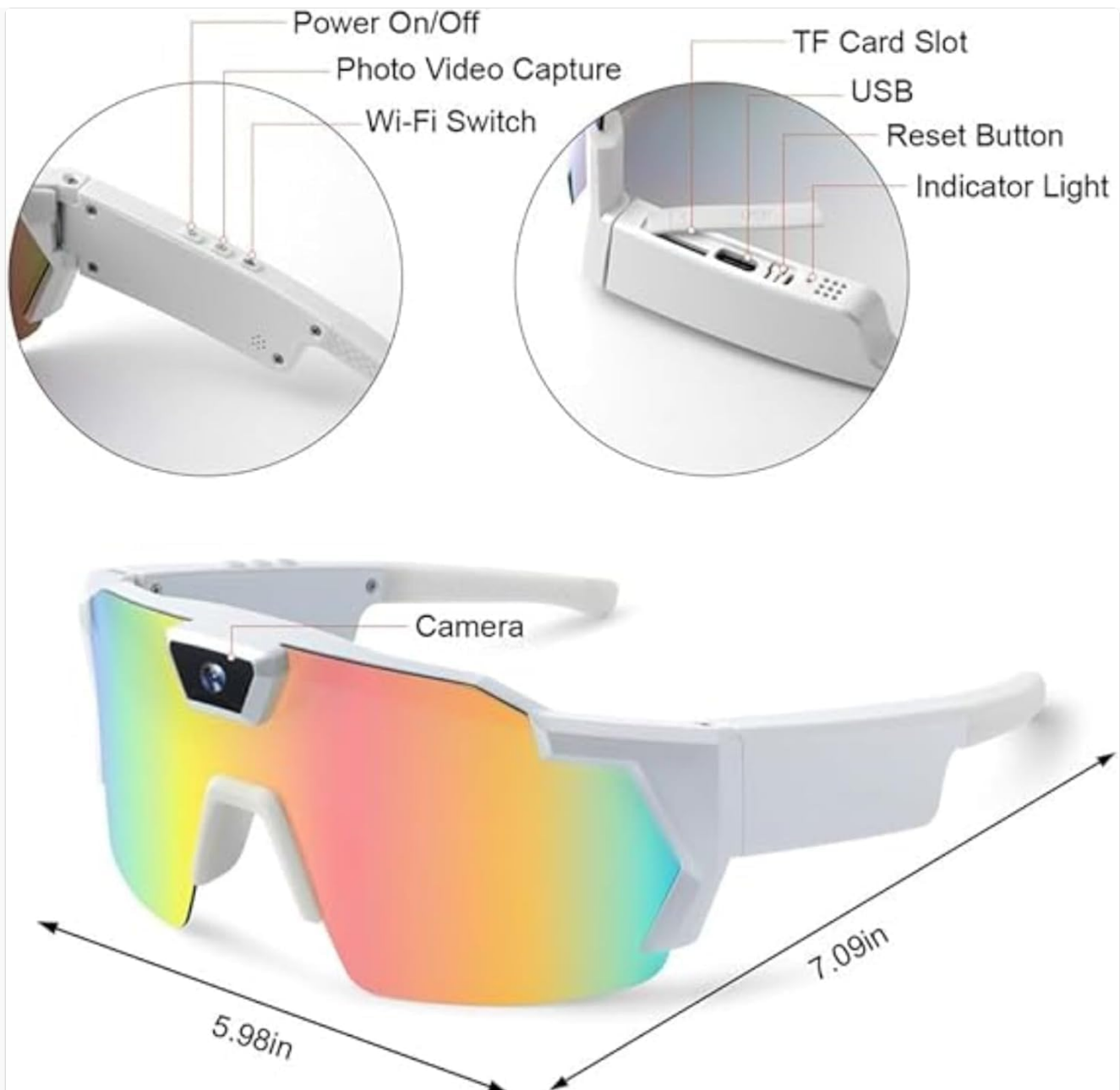
Image 2.1: Diagram showing the various parts of the sports glasses camera, including the Power On/Off button, Photo/Video Capture button, Wi-Fi Switch, TF Card Slot, USB port, Reset Button, and Indicator Light.
